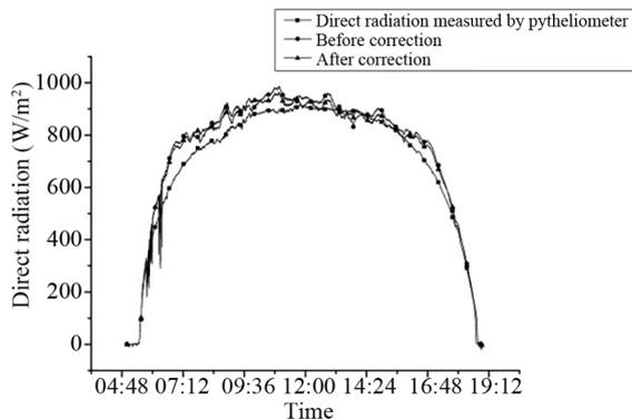
**Fig. 12 Circumsolar radiation correction results**
