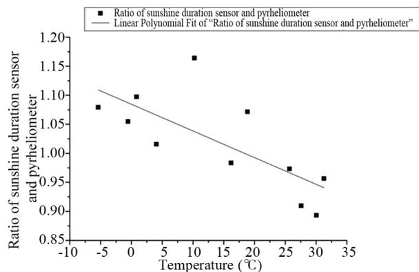
**Fig. 9 Temperature VS error of the direct radiation observation value**
