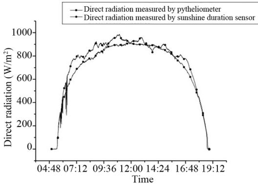
Fig. 5 Actual measured data of Kazuo in sunny days
