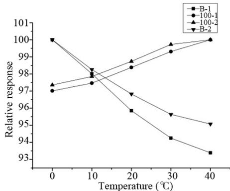
**Fig. 8 Measured result of the temperature characteristics of silicon photodiodes**
