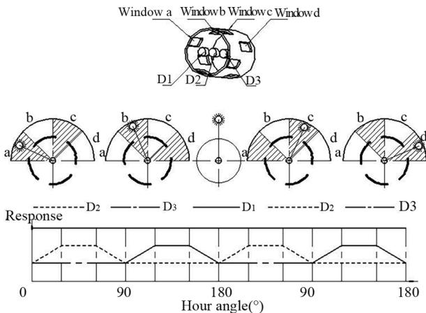
**Fig. 1 Working principle diagram of photoelectric sunshine duration sensor**
