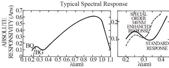
Fig. 11 Spectral response of silicon photodiode
