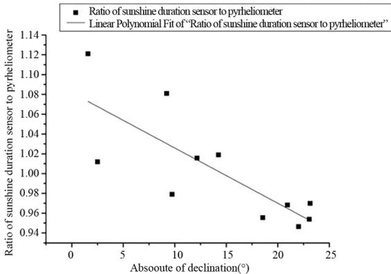
Fig. 6 Declination angle VS direct radiation observational error ratio
