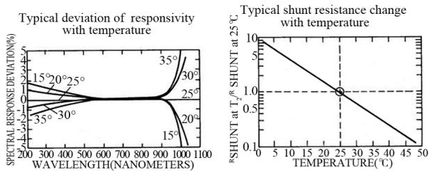
Fig. 7 Temperature characteristics of silicon photodiode
