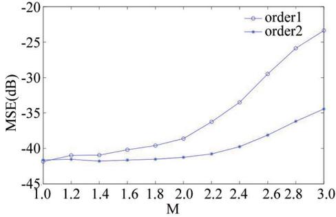
**Fig. 9 MSE of  $\alpha$  of two-component chirp signal under different multiples (  $M = \alpha_1/\alpha_2$  )**
