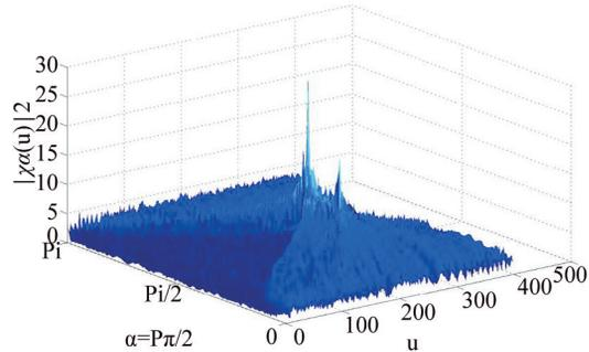
Fig. 7 The energy distribution of the multi-chirp signal
