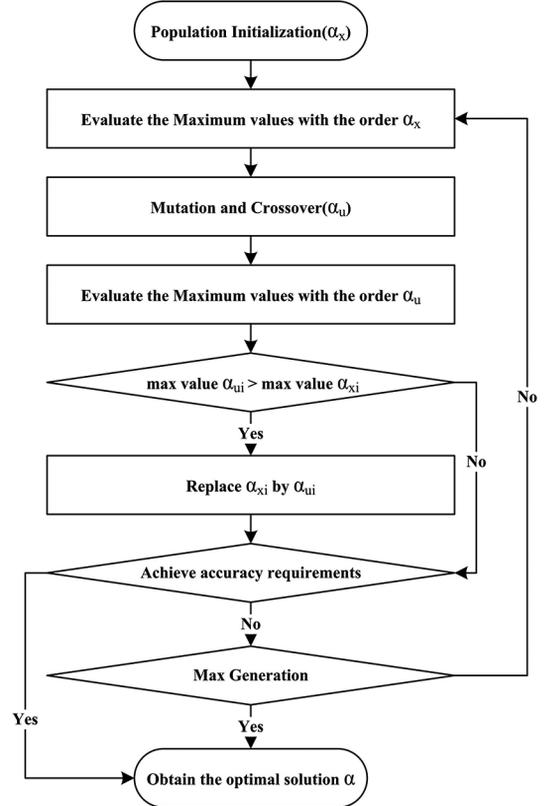
Fig. 2 Flowchart of DE algorithm for single component chirp
