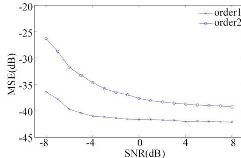
Fig. 8 MSE of  $\alpha$  of two-component chirp signal by rough search
