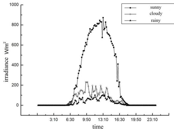
Fig. 7 Daily irradiance changes of solar thermal sensors in different weather conditions
