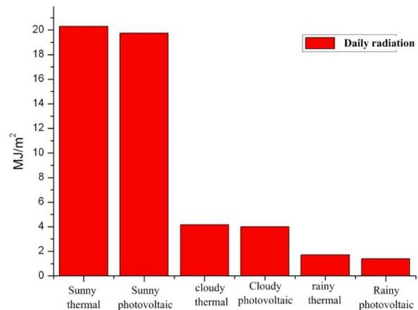
Fig. 9 Daily global radiation changes of solar thermal and photovoltaic sensors in different weather conditions
