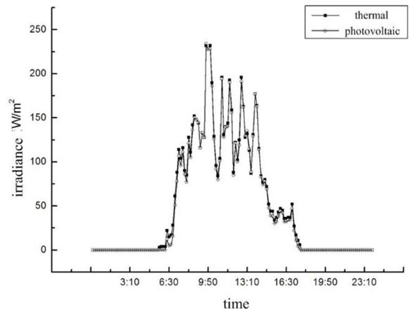
Fig. 5 Daily irradiance changes of solar thermal and photovoltaic sensors in cloudy day
