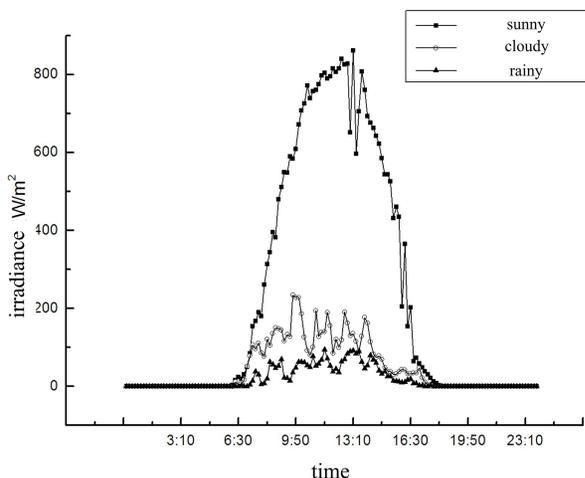
Fig. 8 Daily irradiance changes of photovoltaic sensors in different weather conditions
