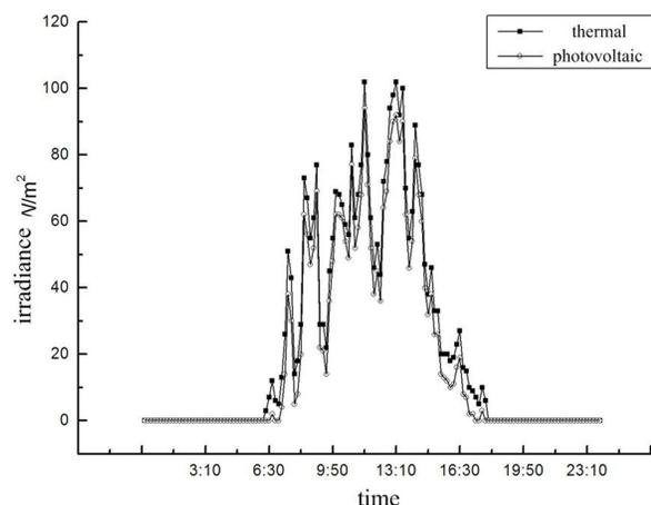
Fig. 6 Daily irradiance changes of solar thermal and photovoltaic sensors in rainy day
