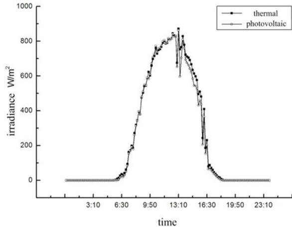
Fig. 4 Daily irradiance changes of solar thermal and photovoltaic sensors in sunny day
