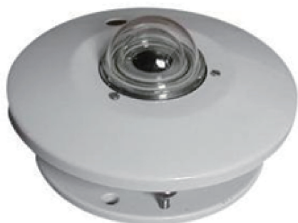
Fig. 3 TBQ-2-B working standard pyranometer
