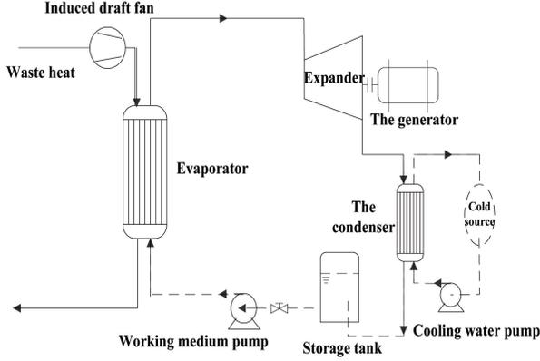
Fig. 1 The principle of ORC
