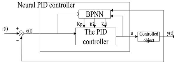
**Fig. 3 Schematic diagram of BP-PID controller**
