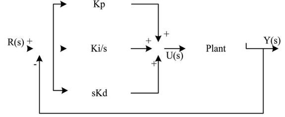
Fig. 2 Schematic diagram of PID controller
