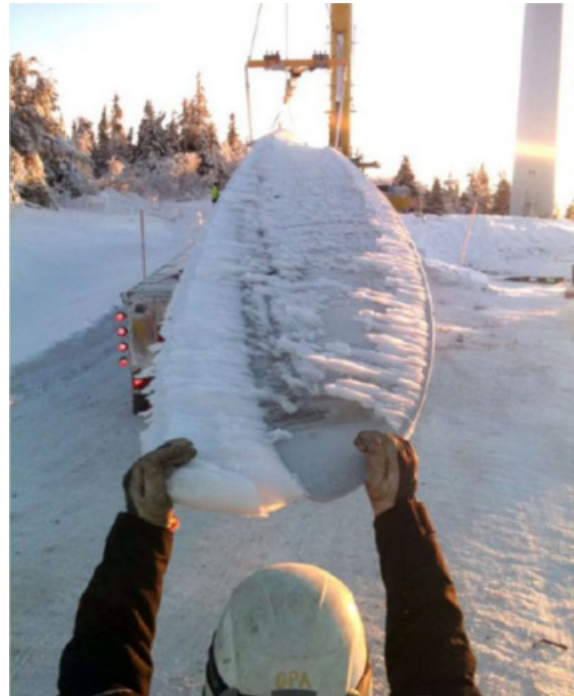
Fig.4 Ice Accretion on a Turbine Blade
