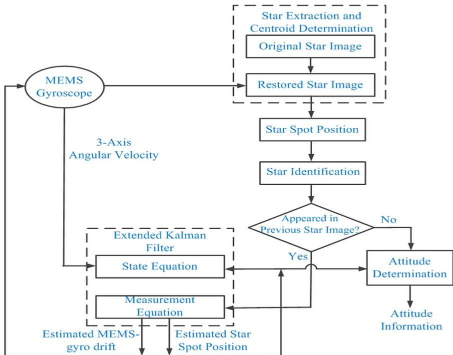
Fig. 6 Flow diagram of deep coupling of star tracker and MEMS-gyro data<sup>[46]</sup>
