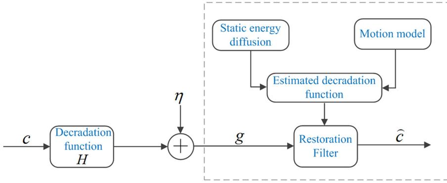
Fig. 7 Degradation and restoration process model<sup>[45]</sup>
