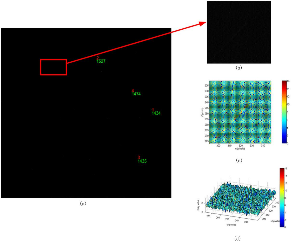
**Fig. 4 Star extraction and recognition results without extra processing method, (b), (c), (d) are gray scale, colour scale and 3D plots of the same detailed view of one star point<sup>[44]</sup>**
