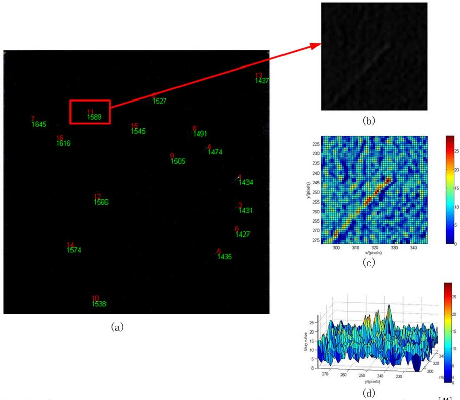
Fig. 5 Star extraction and recognition result with processing method in Reference<sup>[44]</sup>, (b), (c), (d) are gray scale, colour scale and 3D plots of the same detailed view of one star point<sup>[44]</sup>
