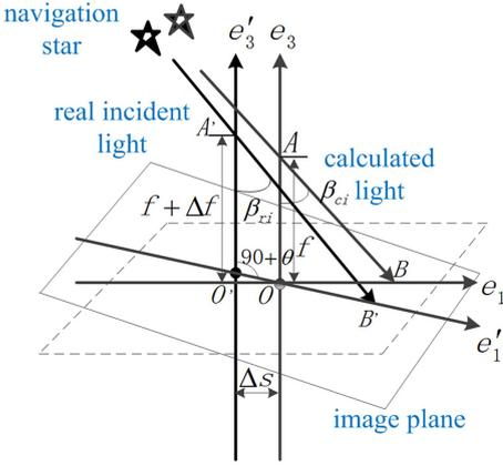
**Fig. 1 Sketch of error propagation model of the star tracker<sup>[43]</sup>**
