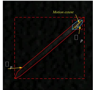
**Fig. 3 The schematic of star extraction and centroid determination with reference window for one star region<sup>[44]</sup>**
