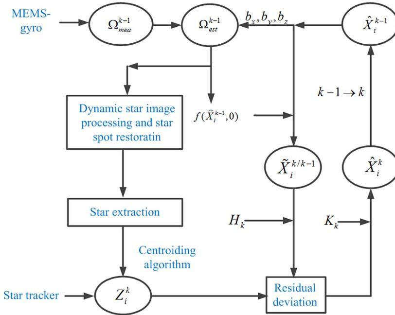
Fig. 8 Flow chart of the deep coupling of star tracker and MEMS-gyro data for determining the position of star spots and gyro drift<sup>[46]</sup>
