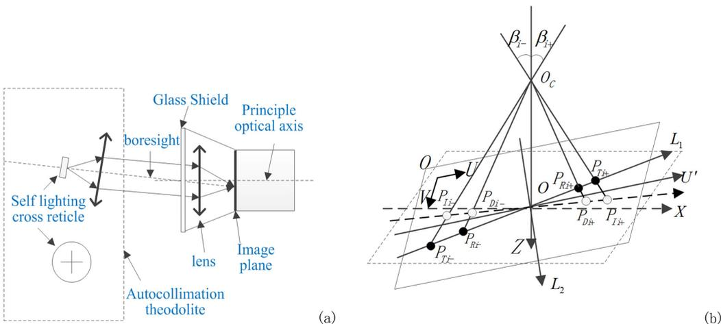
**Fig. 2 Star tracker calibration device (a) and calibration schematic diagram (b)<sup>[43]</sup>**
