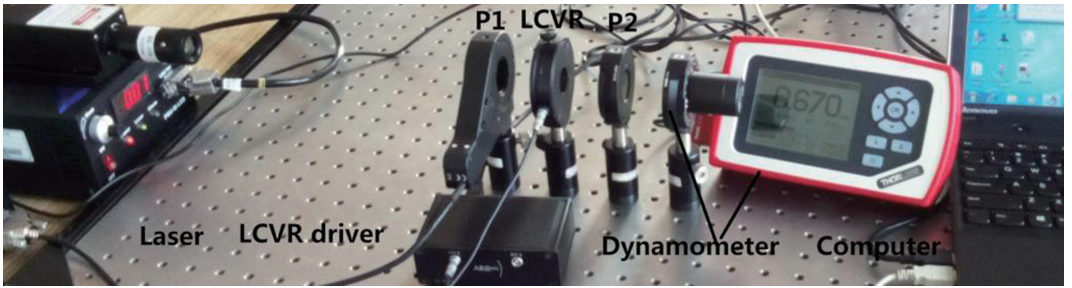
Fig. 1 The experimental Setup of LCVR phase retardance measurement
